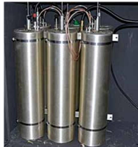
**PHOTO 1:** A typical set of 2m cavity filters.
